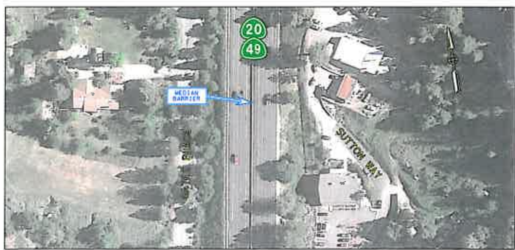
EXAMPLE OF AN EXISTING 22' MEDIAN WITH BARRIER APPROXIMATELY 4 MILES NORTH OF PROJECT IN GRASS VALLEY ON HIGHWAY 20/49 WITH FRONTAGE ROADS
